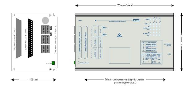
The **AMG5903A966** is a standalone data transmit unit designed to transmit and receive 2 data channels, 6 audio channels, 2 Echelon FTT-10A data channels and 8 bi-directional alarms over one Singlemode optical fibre. It also provides full duplex 100Base-T Ethernet connectivity.
